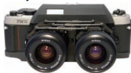
A modern RBT custom-built camera made by cutting and joining two SLRs
